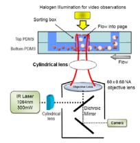
Fig. 2: Schematic of optical sorting microfluidic system with focused laser applied at the junction of the two overlapping channels
